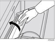
**3** Remove the used master roll and pull out both spools. Then, insert both spools into a new master roll.
